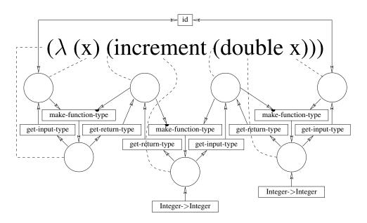
Figure 5-14: A complete sample type inference network
