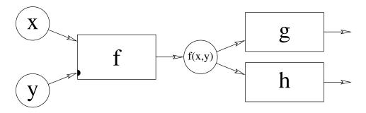
Figure 2-1: A sample fragment of a propagator network. Information about x and y has just propagated through f; now g and h have an input they can work on. The black semicircle marks y as the second argument of the (presumably noncommutative) function f.
