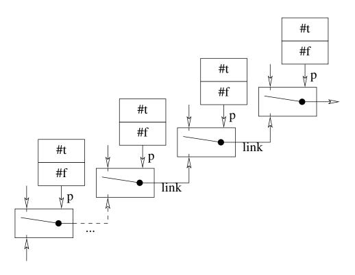
Figure 4-6: A linear chain turning binary guessers into an n-ary guesser. It consists of binary-amb boxes, drawn as in Figure 4-4, and conditional boxes, to be defined carefully in their own Section 6.1, and drawn as in Figure 6-4 on page 112.
