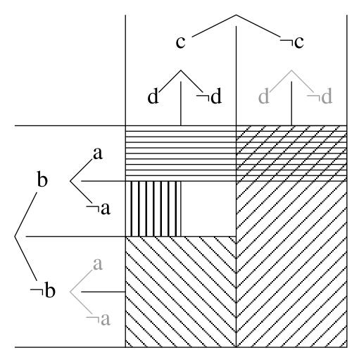
Figure 5-4: A search hypercube. Discovered nogoods can eliminate large chunks of the cube at once: Each of the nogoods  $\{a,b\}$ ,  $\{\neg b,c\}$ ,  $\{\neg c\}$ , and  $\{\neg a,b,c,d\}$  is indicated with its own shading.
