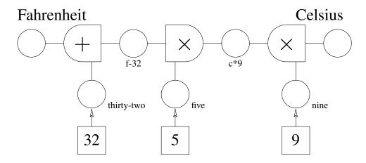
Figure 3-4: A multidirectional temperature converter. Now the + and  $\times$  boxes each look like Figure 3-3 inside, and can compute in whatever direction the available data permits. That's why they don't have arrowheads on their connections.
