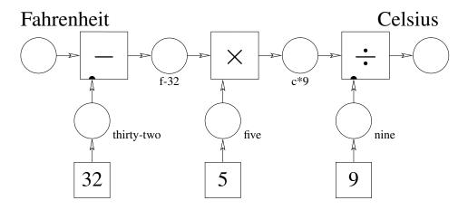
Figure 3-1: A Fahrenheit to Celsius converter network
