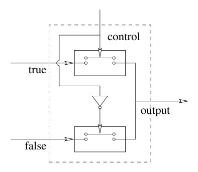
Figure 6-3: A conditional made out of switches
