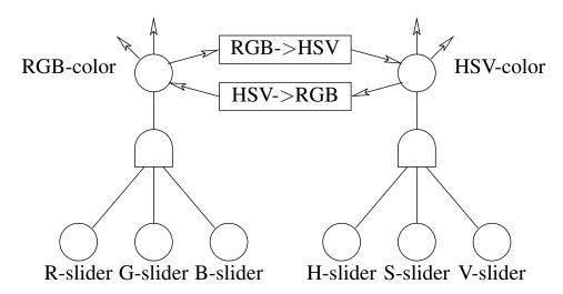
Figure 5-8: A network for a widget for RGB and HSV color selection. Traditional functional reactive systems have qualms about the circularity, but general-purpose propagation handles it automatically.
