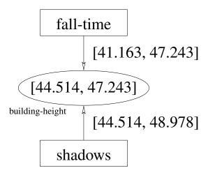
Figure 3-6: Partial answers from different sources merge at a cell. The merged result incorporates all the information available in both partial results.
