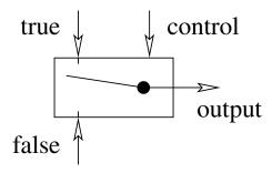
Figure 6-4: Conventional diagram of a conditional
