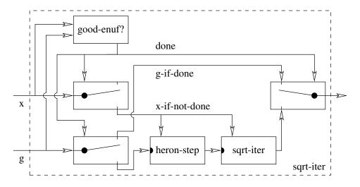
Figure 6-8: The recursive sqrt-iter network
