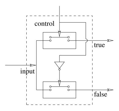
Figure 6-6: A conditional-writer made out of switches. Note the symmetry with the conditional in Figure 6-3.
