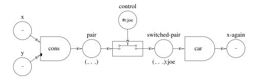
Figure 6-10: A propagator network with a cons and a switch
