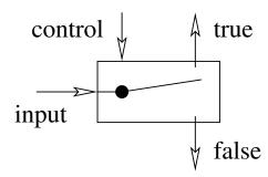
Figure 6-5: Conventional diagram of a conditional-writer
